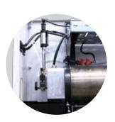
Output pressure transducers activate the discharge module to avoid overpressure on the system
